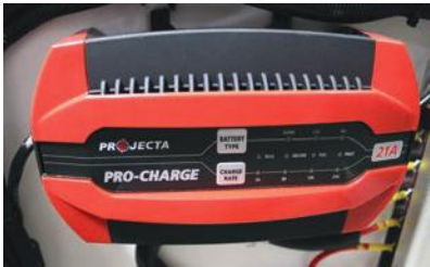
Batteries 2x 100Ah deep cycle AGM batteries with 240V charger
